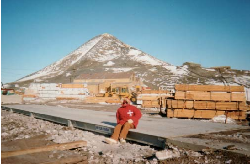
METTLER TOLEDO scale installed at McMurdo Station, the only truck scale in Antarctica (Average temperature -17^{\circ}\text{C} )
